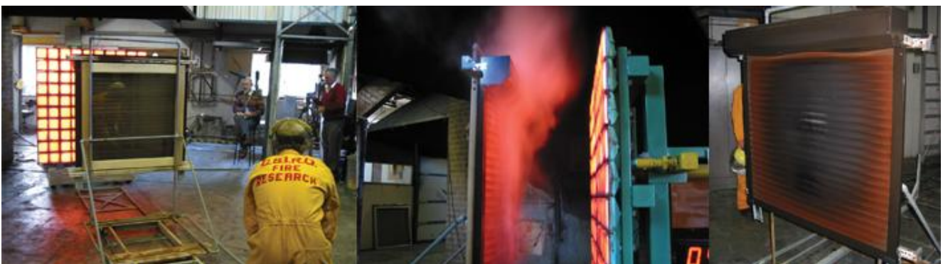
CSIRO – Bushfire Simulation Testing on OZRoll® shutter profiles
