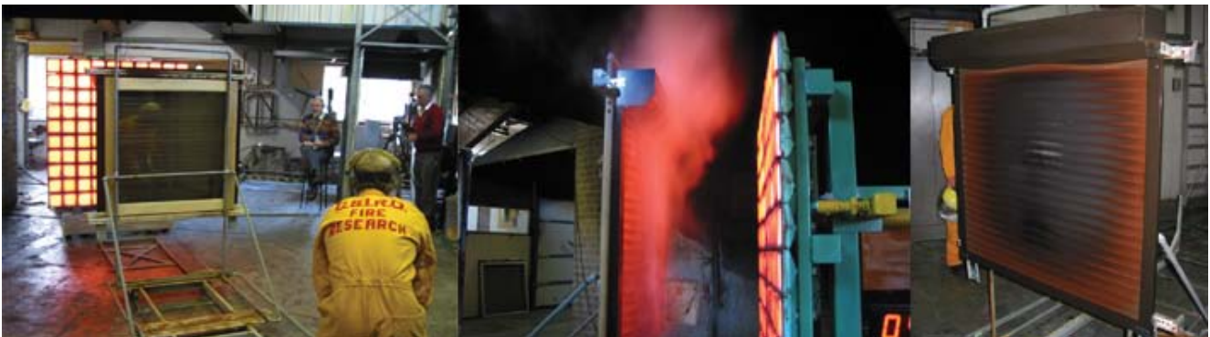
CSIRO – Bushfire Simulation Testing on OZRoll® shutter profiles
